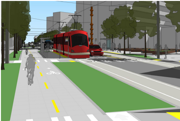
Above: Seattle's First Hill Streetcar will feature separated bike lanes in the same right-of-way. Image credit: Seattle Department of Transportation.
